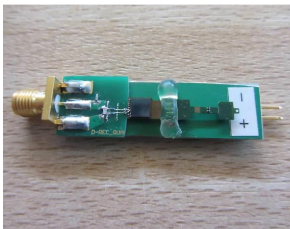
PCB with temporary antenna & supply connectors (for § 7.4 test)
