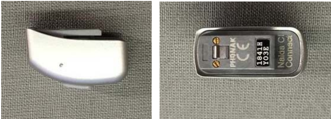
Naída CI Connect – brand and product name are placed on the short side of the battery compartment.
