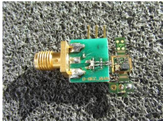
D-Receiver's radio module with temporary antenna & supply connectors (for § 7.4 test)
