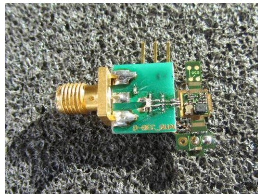
Electronic board with temporary antenna &amp; supply connectors (for § 7.4 test)
