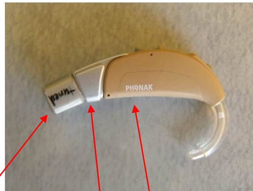
MLxD plugged onto battery holder of Ambra SP/AS13 hearing aid
