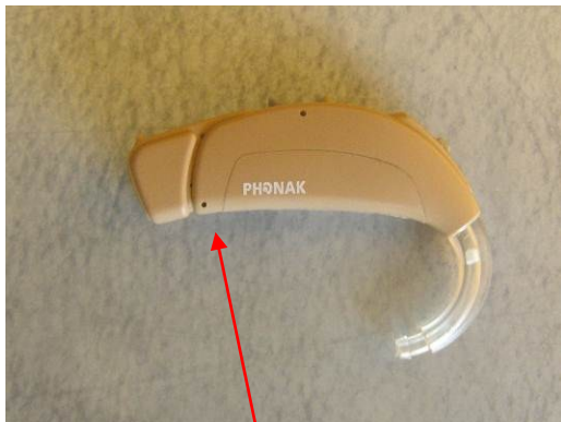
ML13D implemented inside battery holder of Ambra SP hearing aid
