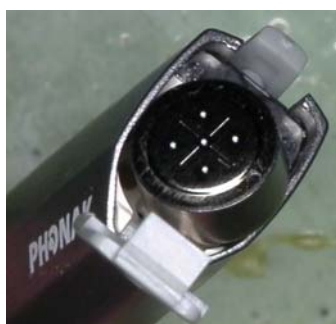
fig. 1a, b, c Zinc Air battery insertion for the BICROS CTX
