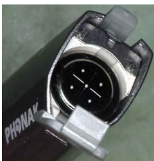
fig. 1a, b, c Zinc Air battery insertion for the BICROS CTX
