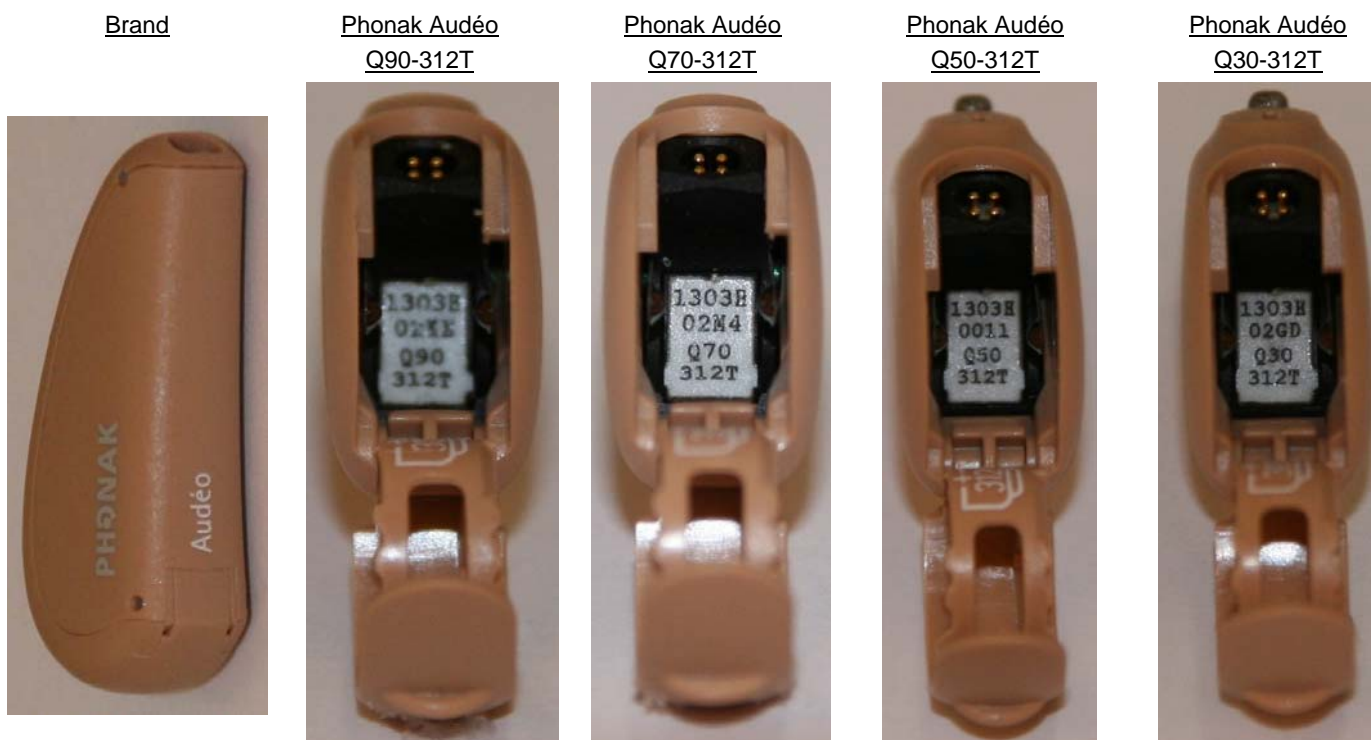
Figure 2a: Phonak Audeo Q hearing aid with a visible brand name on the housing; and a serial number and model number affixed on the battery compartment (current serial number size is 2.2 points).
