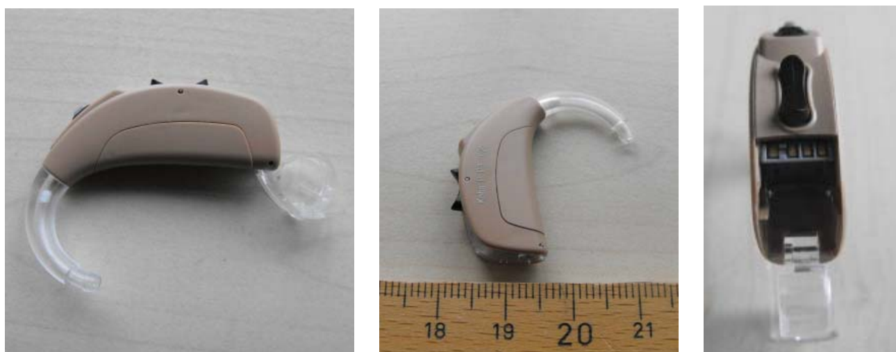
Figure 2: Phonak Ambra P - battery compartment, current serial number size is about 2 points
