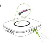
1. Firmly press the on/off  $\circlearrowleft$  button or the mute on button on the remote control to mute Roger Table Mic's microphone or audio input.
