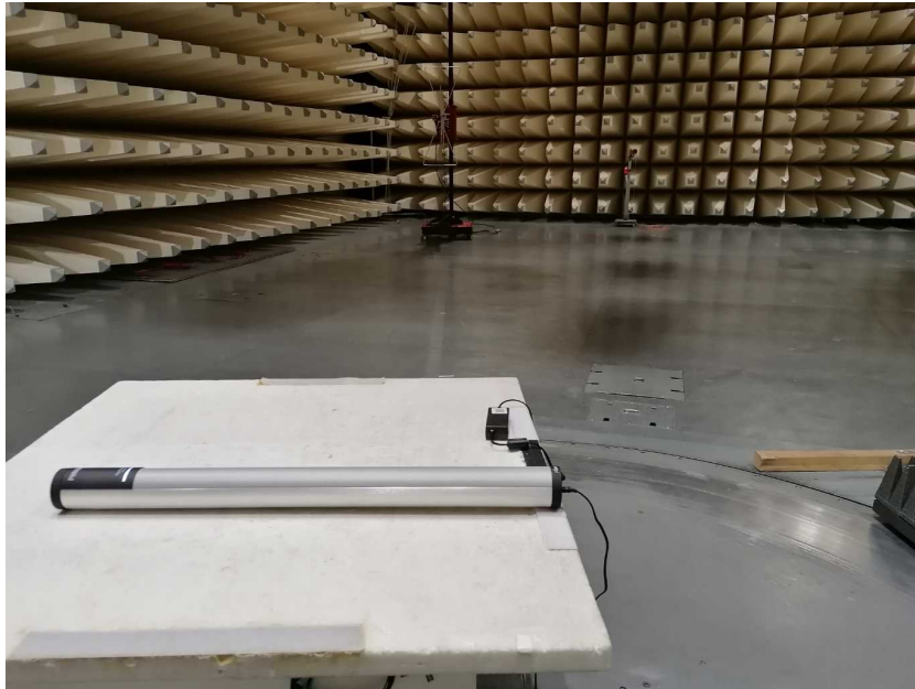
Photo 7: EUT at the semi-anechoic chamber
