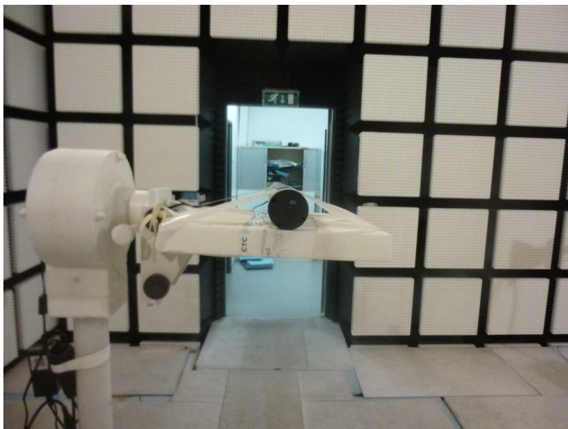
Photo 4: EUT at the anechoic chamber
