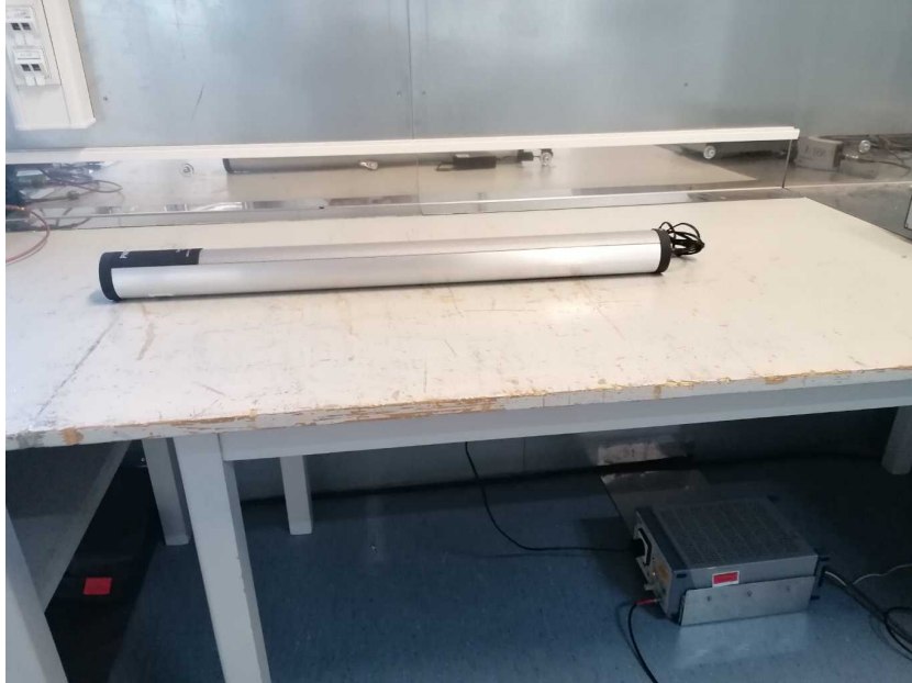
Photo 9: AC conducted emission test setup
