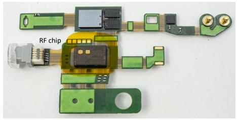
picture of the antenna PCB Audeo I-Sphere The antenna PCB is externally sourced and there are no components on it.
