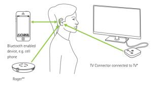
\* The TV Connector can be connected to any audio source such as a TV, PC or hi-fi system. \*\* Roger wireless microphones can be connected to your hearing aids as well.
