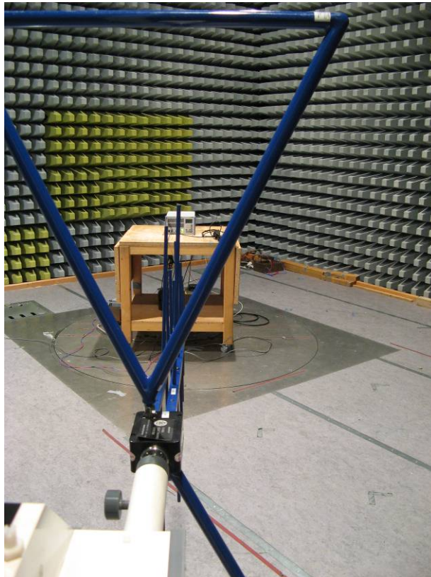
Figure 6-1: Test setup for radiated emission measurement, 30
