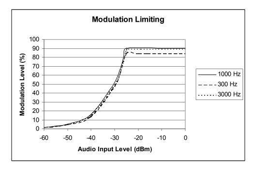
FCC PART 87, SUBPART D PROJECT NO.: 3W06782 EQUIPMENT: VHF Transceiver
