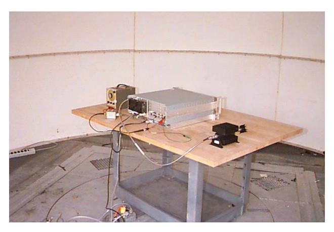
TX 128 MHz, 30 Watts Modulated 2500 Hz, 16 dB overdrive (ref: 50% modulation, 1000 Hz)
