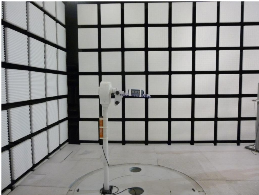
Photo 3: Fully anechoic chamber
