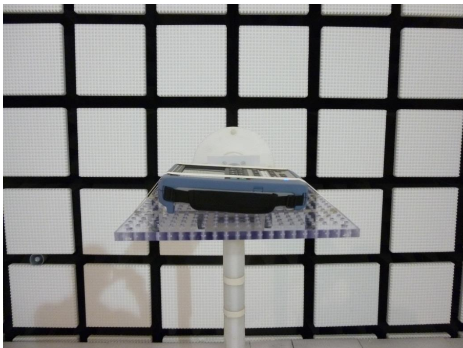
Photo 5: Fully anechoic chamber
