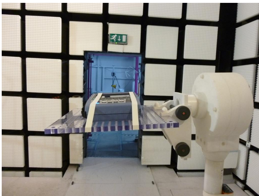
Photo 6: Fully anechoic chamber
