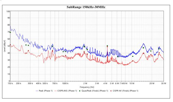
Phase 1, UWB and digital circuitry for UWB generation OFF
