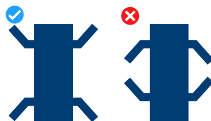
Figure 4-4: Correct alignment of the supporting feet
