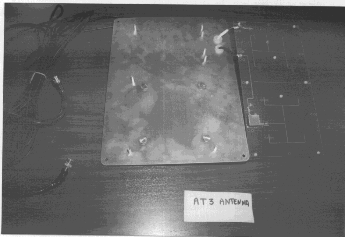
8-20 AT3 antenna inside (continued)
