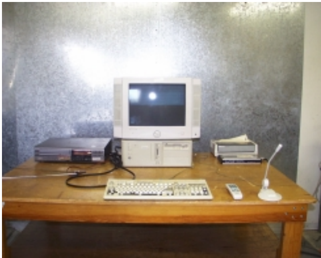
Conducted Emission Setup Photos (Worst Emission Position)
