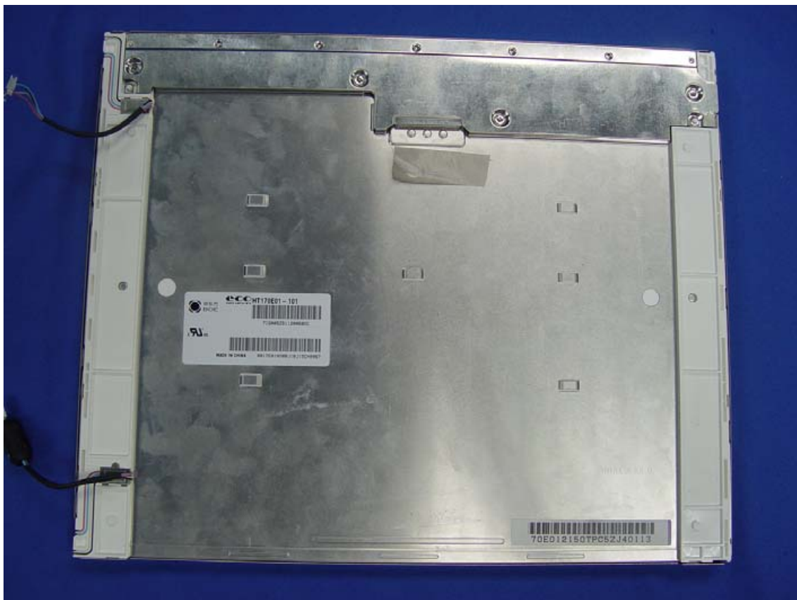
Figure 10 Backside of the LCD Panel
