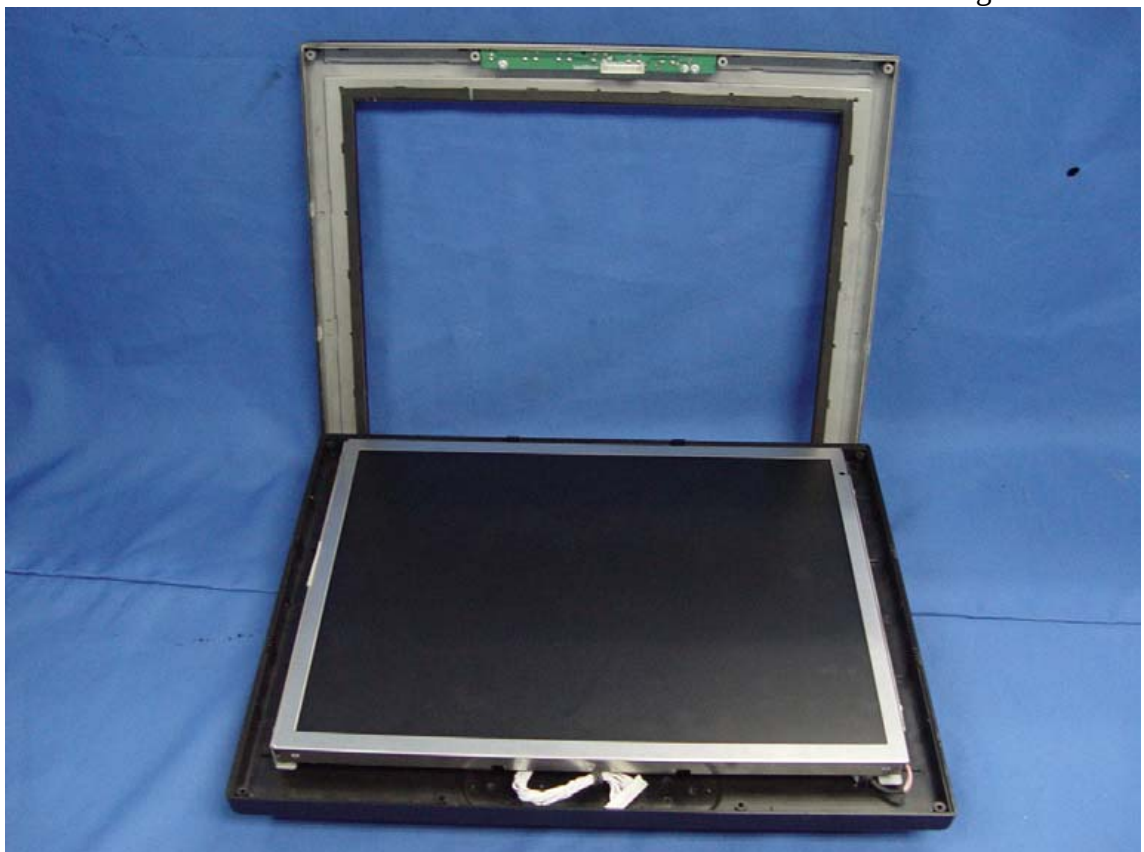
Figure 6 Inside Configuration of the EUT
