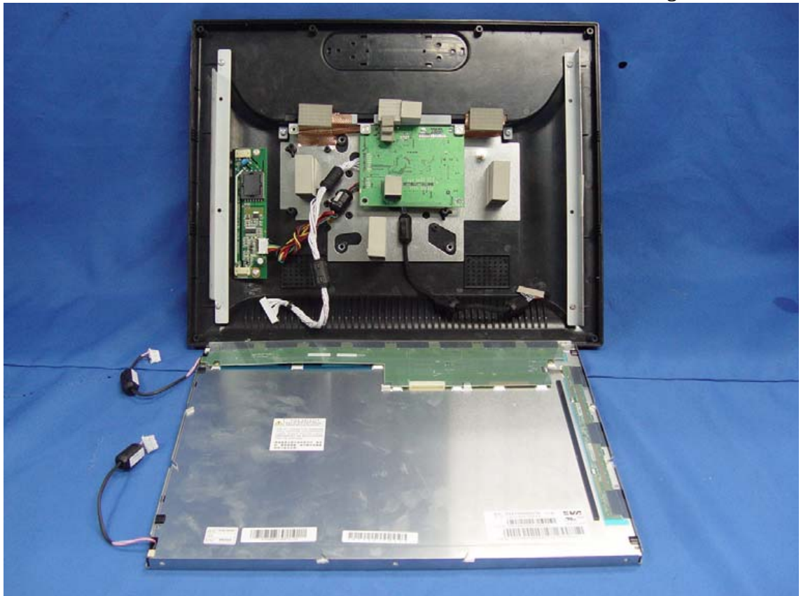
Figure 7 Inside Configuration of the EUT
