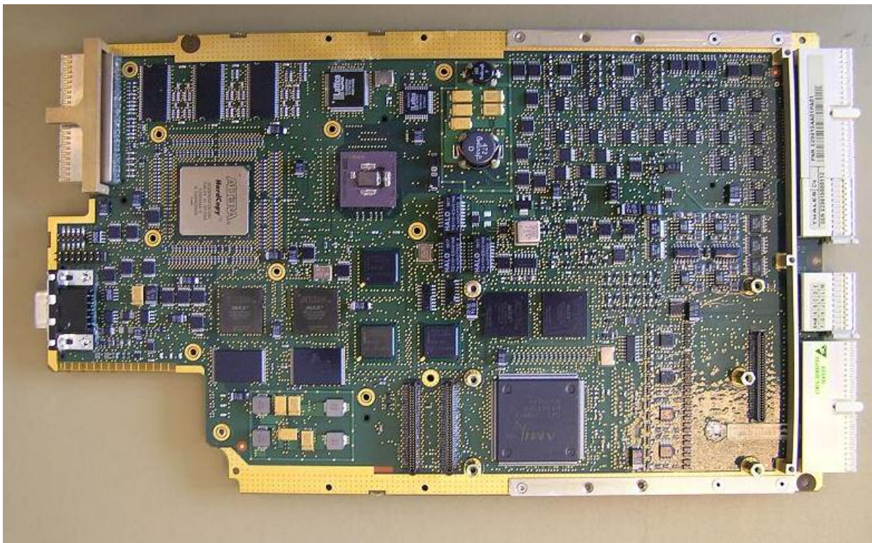
Figure 2: SDU Avionics Processor Module (APM) Top. With Heatsink Removed.
