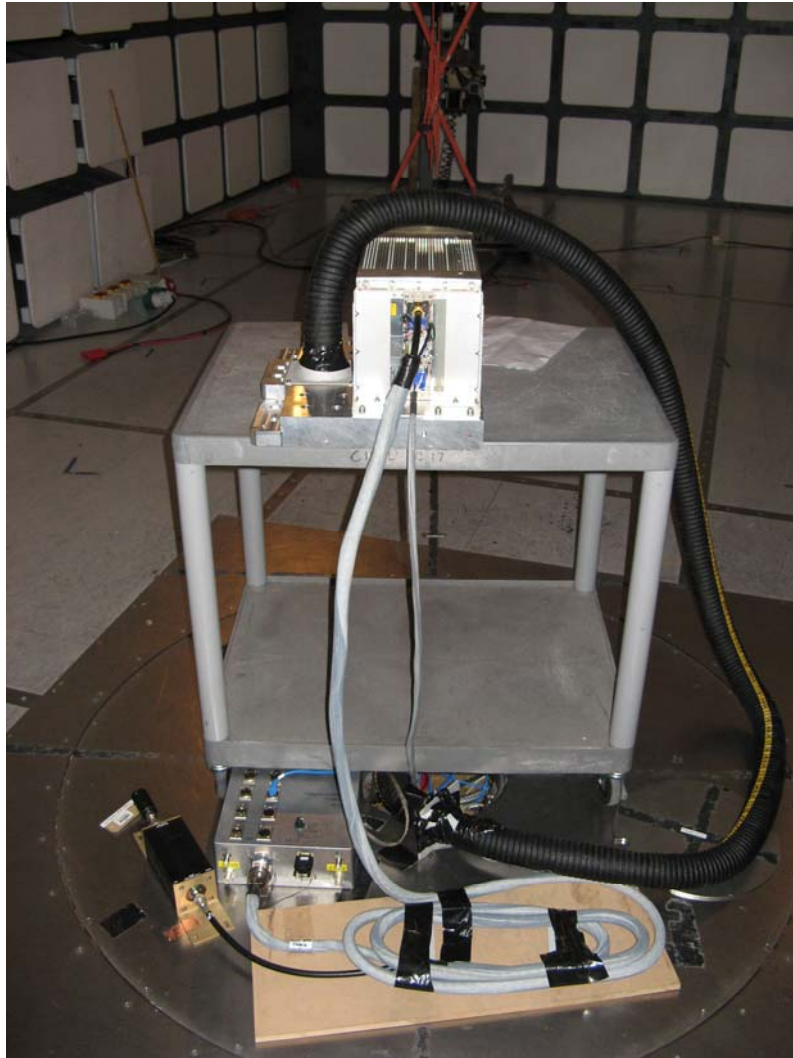
Radiated Emissions Test Setup
