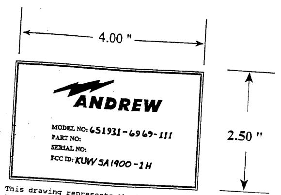
This drawing represents the label that will be affixed to the rear of the amplifier case. This label will printed on a mylar material which has been selected to last the life of the product.
