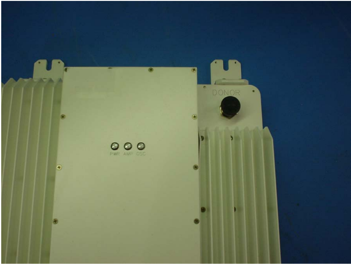
Figure 7. Detail Showing Indicator LEDs on KUWR1900L
