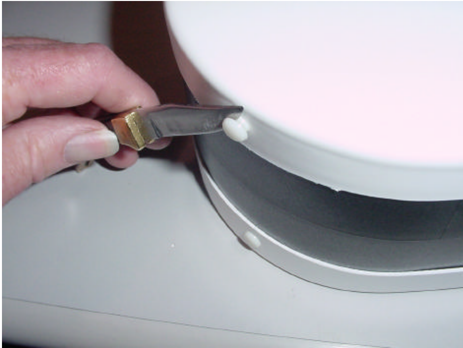
Figure C-1. Plastic Rivet Staking Pin Removal
