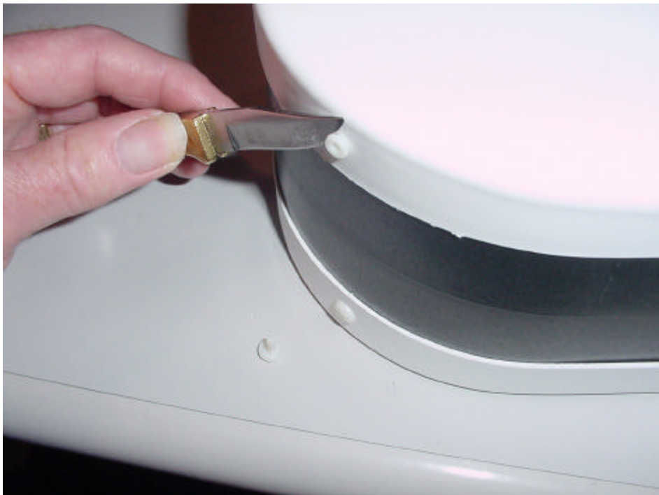
Figure C-2. Plastic Rivet Expansion Sleeve Removal
