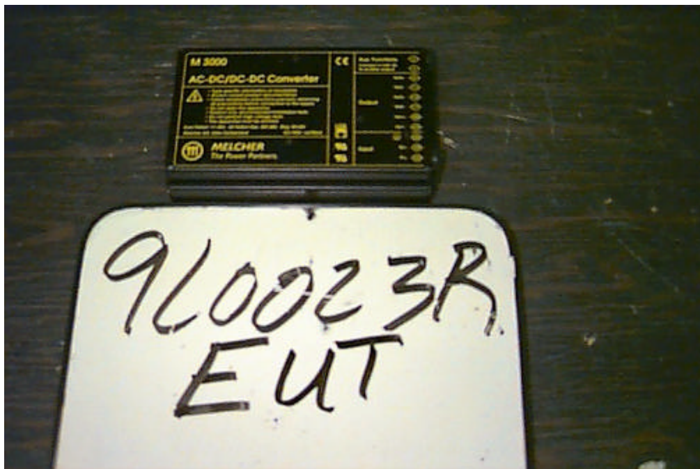
Photo 19 - AC/DC converter module
