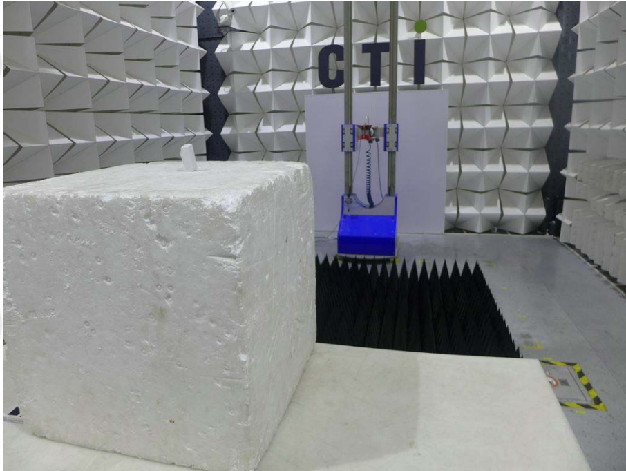
Radiated spurious emission Test Setup-3 for GS-MT2(Above 1GHz)
