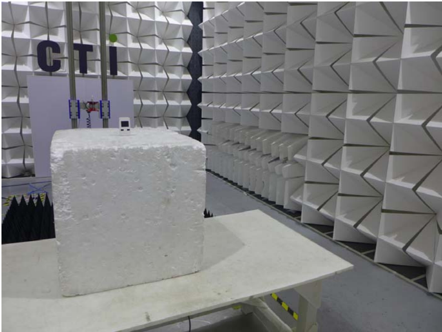
Radiated spurious emission Test Setup-4 for WB-630(Above 1GHz)
