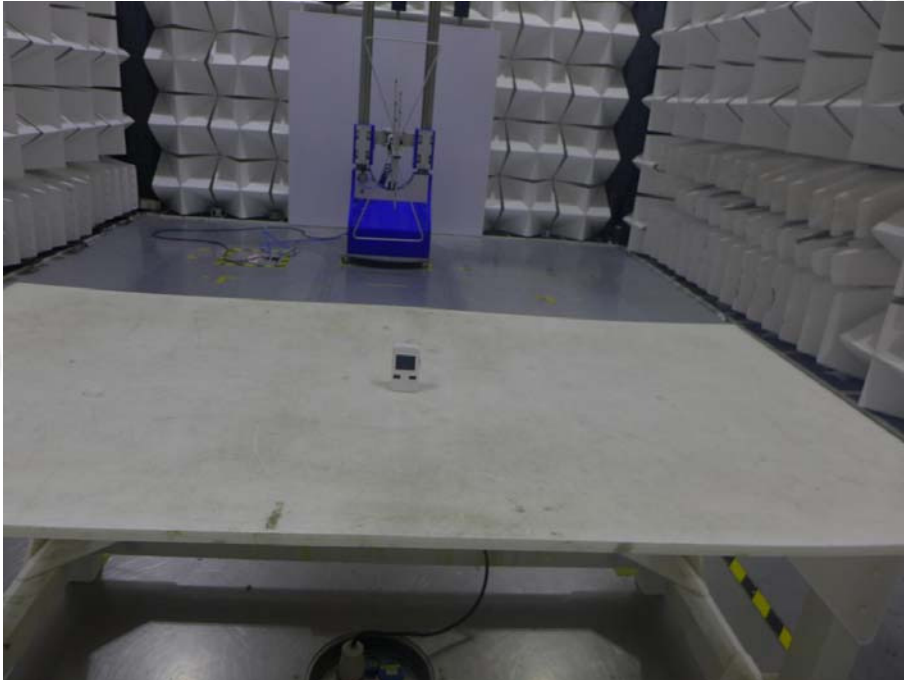
Radiated emission Test Setup-1 for WB-660(30MHz~1GHz)
