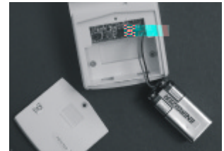
Insert 9V alkaline battery to the sensor
