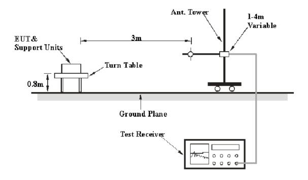
The deactivation test was performed in the 3 meters chamber B test site, using the setup accordance with the ANSI C63.4 - 2009. The specification used was the FCC 15.231(a) limits.
