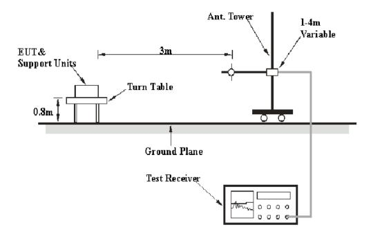
The radiated emission tests were performed in the 3 meters chamber B test site, using the setup accordance with the ANSI C63.4 - 2009. The specification used was the FCC §15.209 and §15.231.
