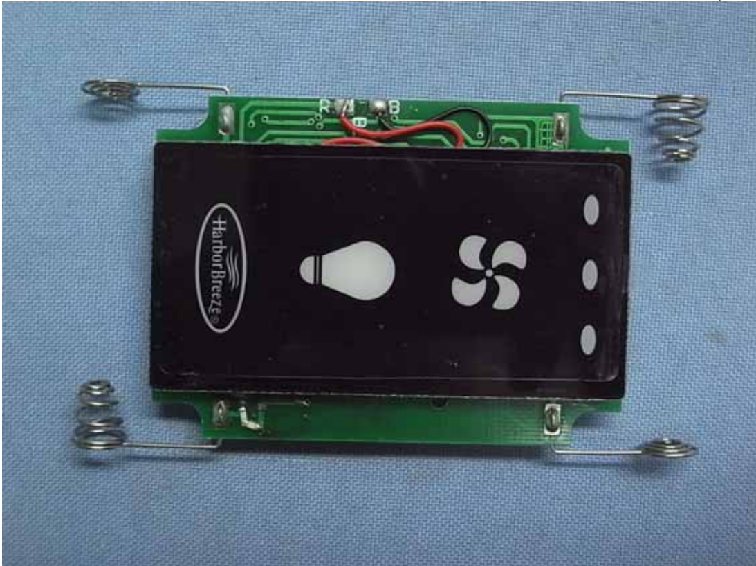
Photo 5 PCB View (Front Side)
