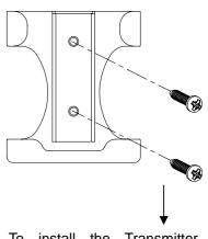
To install the Transmitter Wall Mount Holder with two screws.
