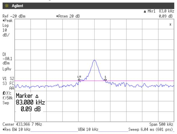
Note: "\$" The line is 20dB from the modulated carrier.
