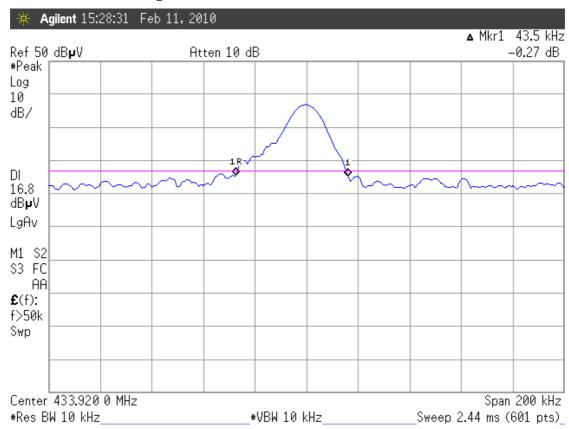
Note: "\odot\" The line is 20dB from the modulated carrier.
