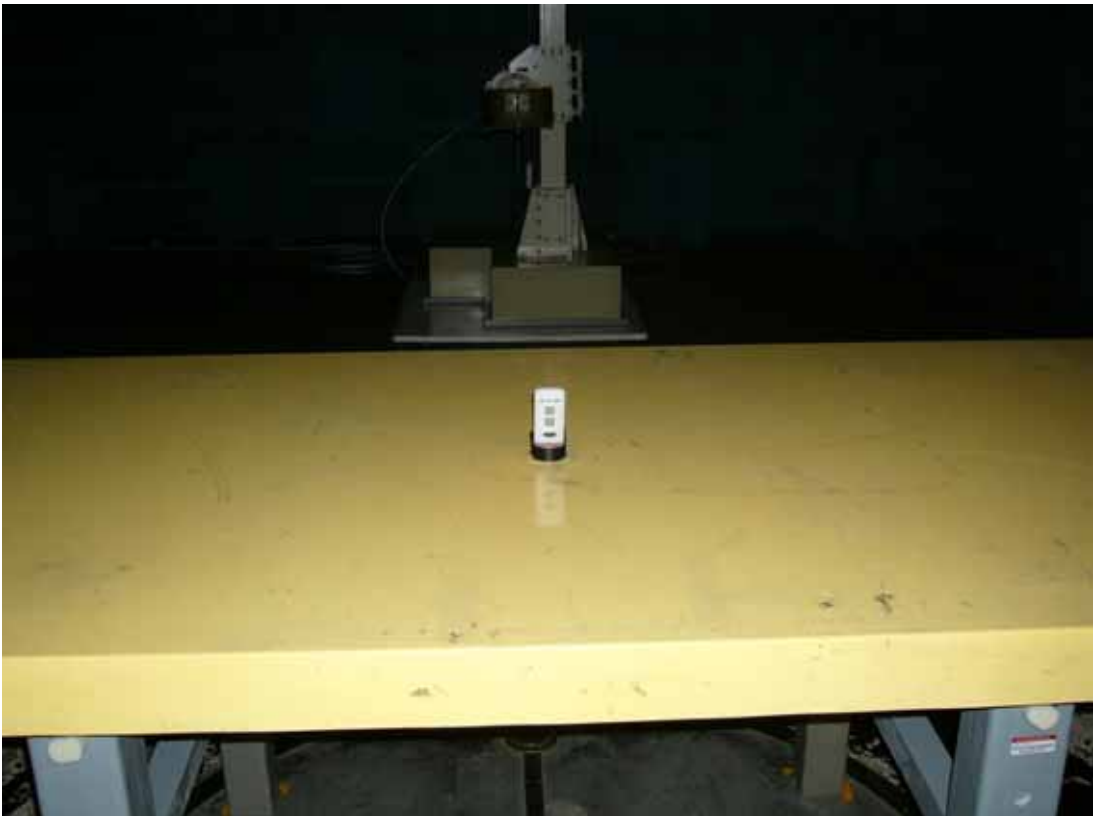
7.2. Photos of Radiated Measurement at Semi-Anechoic Chamber (Above 1GHz) Stand Position
