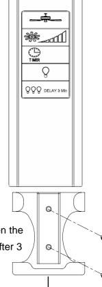
Installation of Transmitter Wall Mount Holder with two screws.
