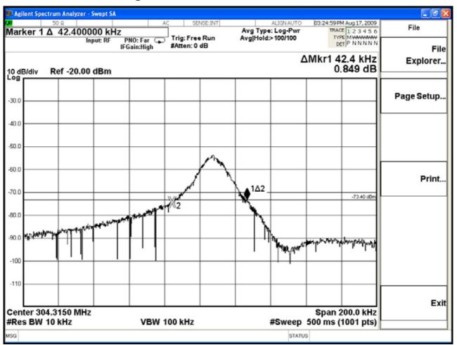
Note: "\$\dangle\$" The line is 20dB from the modulated carrier.
