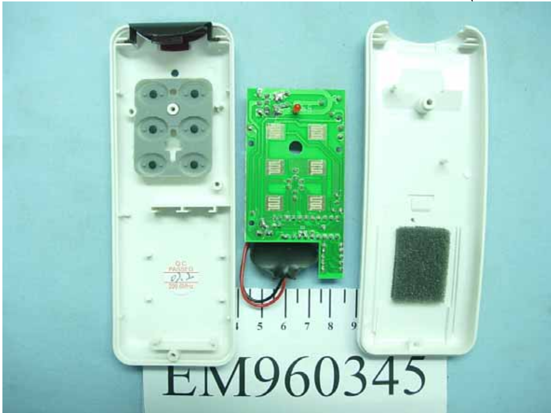
Photo 3 Internal View (Covers Removed)
