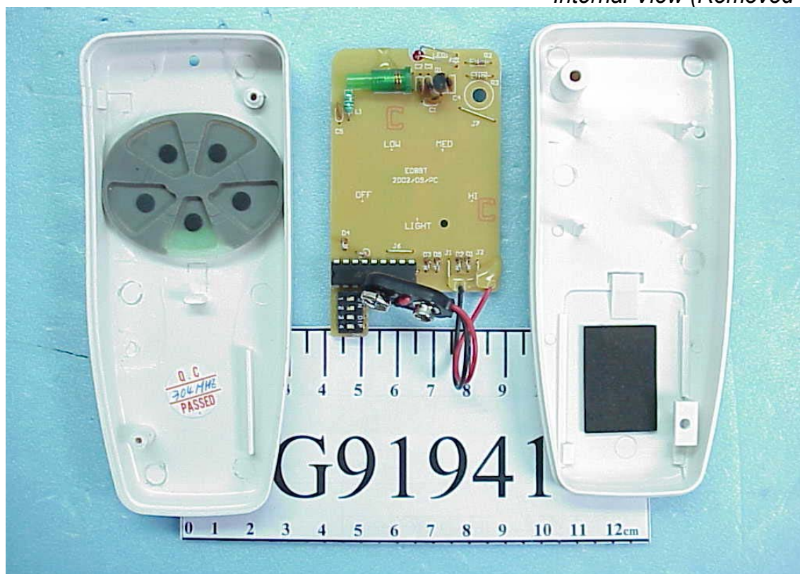
Photos 4 PCB View (Component Side)
