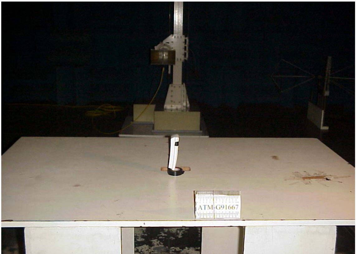
7.2. Photos of Radiated Measurement at Semi-Anechoic Chamber (1~3GHz) EUT on Stand
