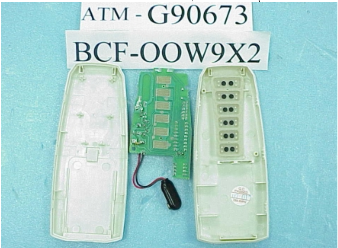
BCF-00W9X2, Internal View (Removed Case Covers)
