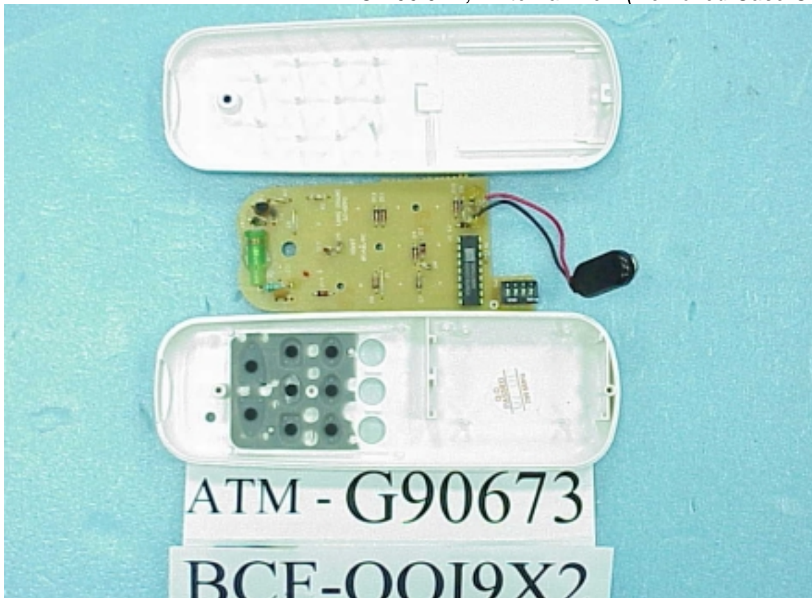
Photos 4 BCF-0019X2, Internal View (Removed Case Covers)
