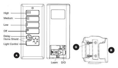
Installation of Transmitter Wall Mount Holder with Two screws
