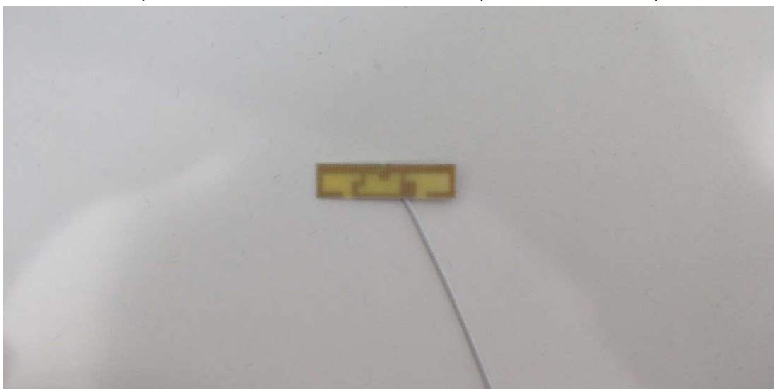
Figure 14 Internal View (WIFI Second Source Antenna (P/N: 290-80076), Front View)
