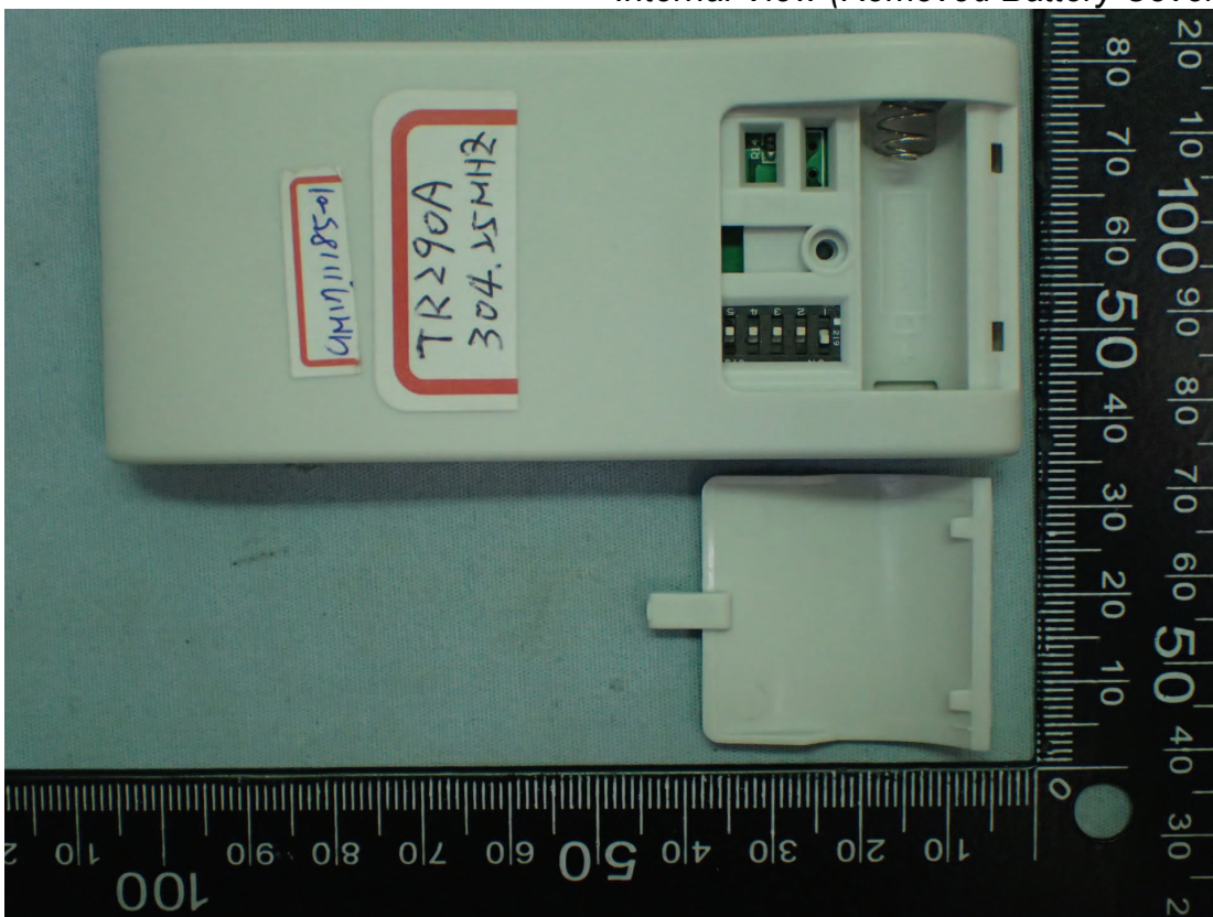
Figure 3 Internal View (Removed Battery Cover)
