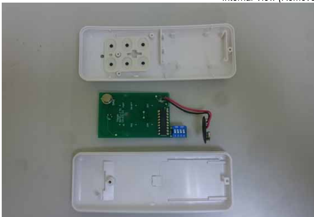
Photo 4 Internal View (Removed Cover)
