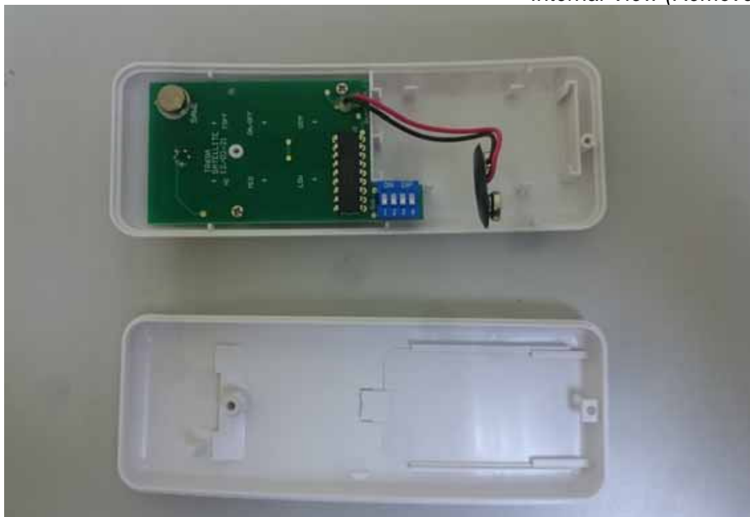
Photo 3 Internal View (Removed Cover)
