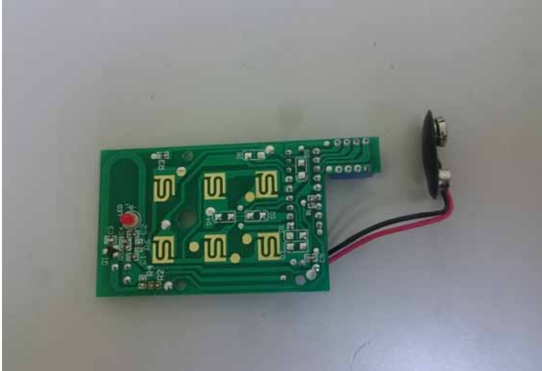
Photo 5 Internal View (Main Board, Front View)
