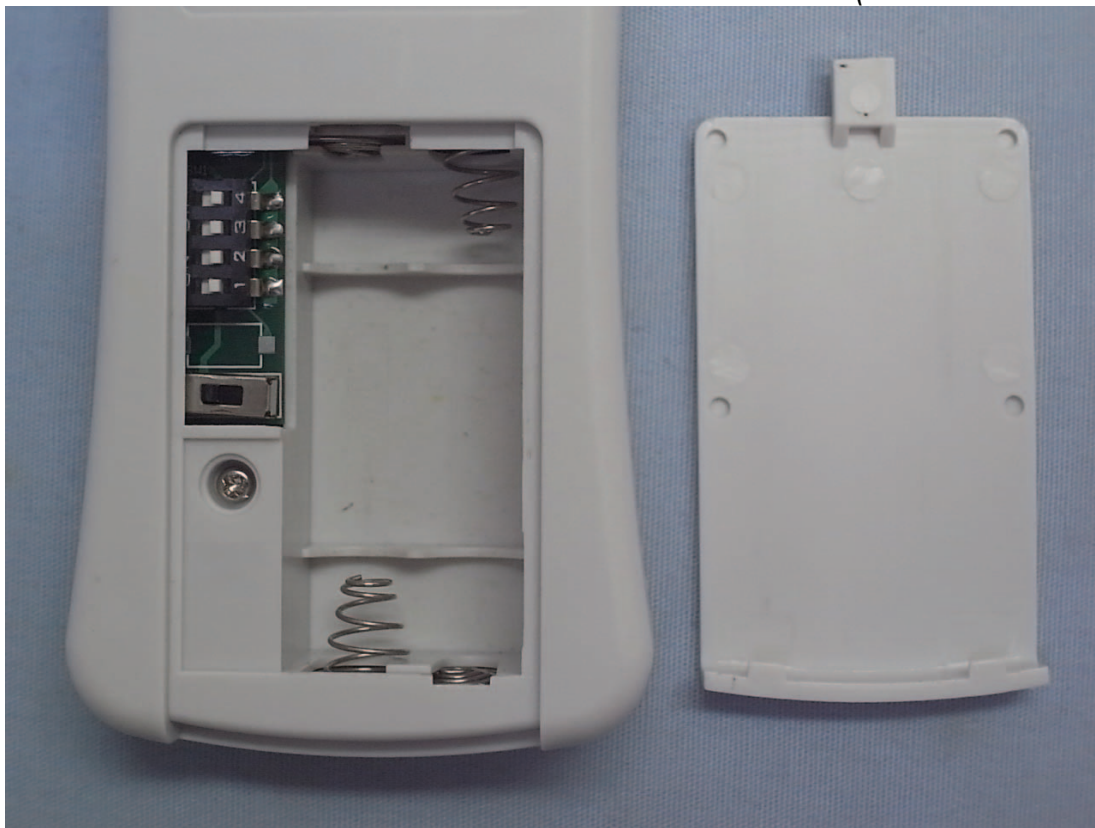
Photo 3 Internal View (Removed Battery Cover)
