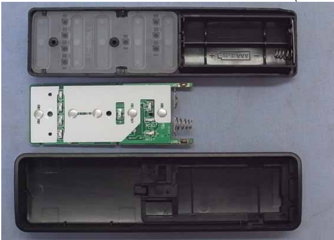
Photo 4 Internal View (Removed Cover)
