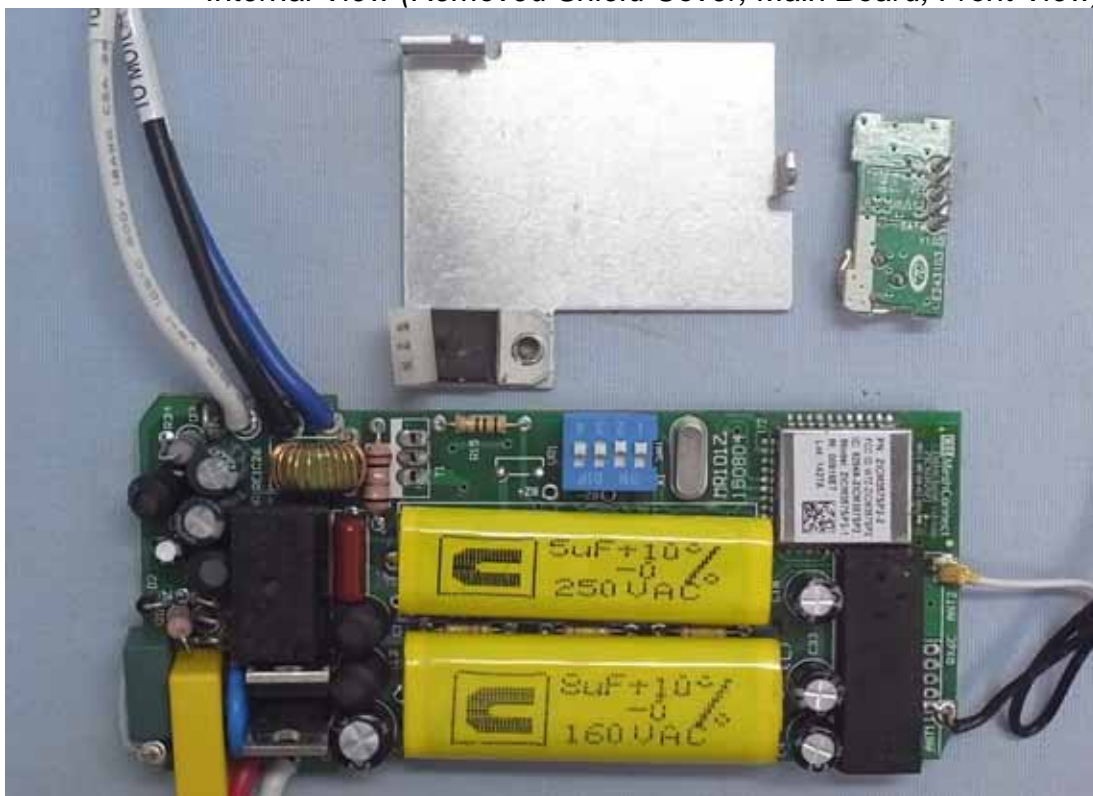
Figure 5 Internal View (Removed Shield Cover, Main Board, Front View)
