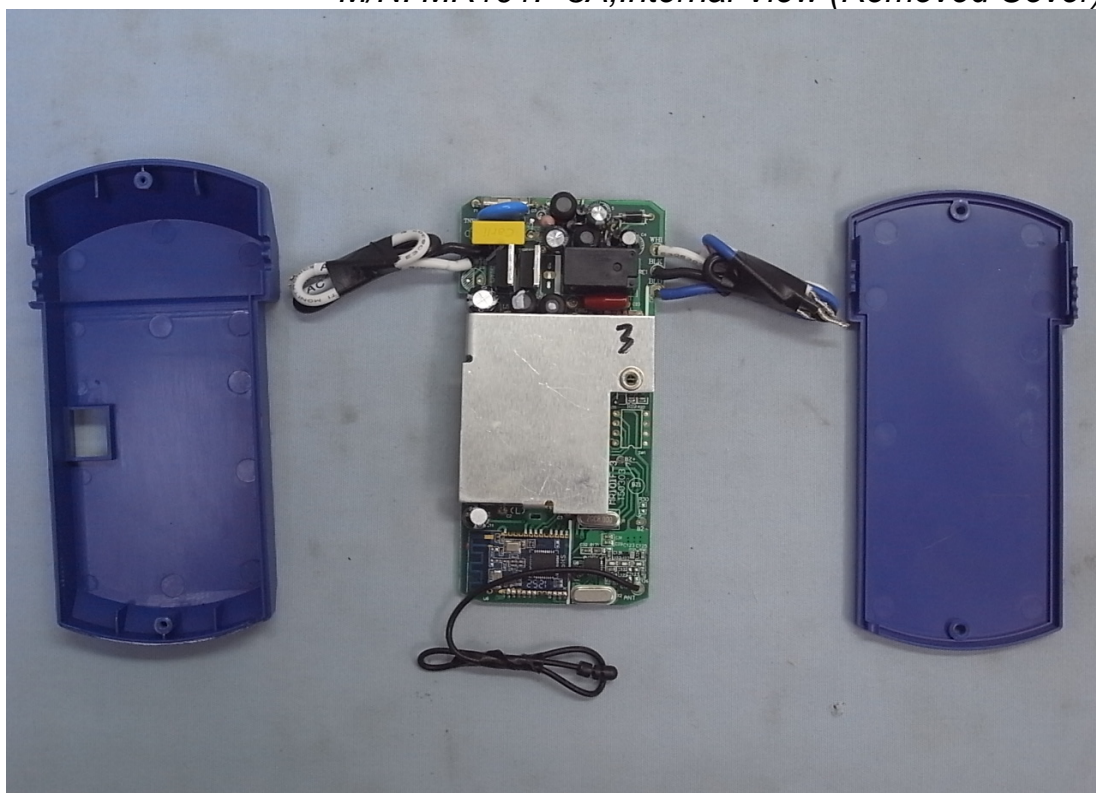
Figure 6 M/N: MR101F-3A, Internal View (Removed Cover)
